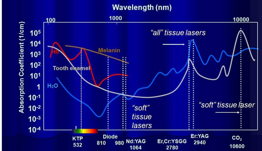
Figure 5. Four absorption curves of the principal dental tissue components. The absorption coefficient in a logarithmic scale is on the vertical axis, and the dental laser wavelengths are on the horizontal axis in ascending order of wavelength.
