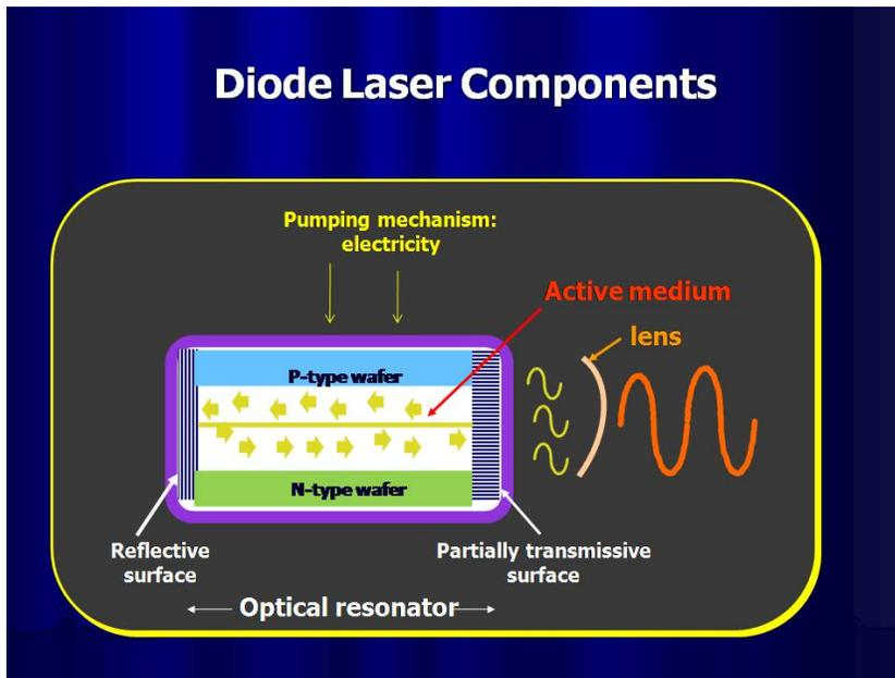
Figure 3 Schematic of a diode laser
