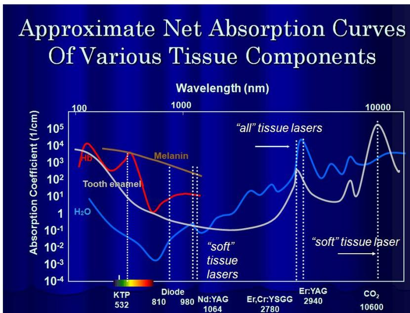
The currently used dental lasers are depicted on the Electromagnetic spectrum, figure 5.
