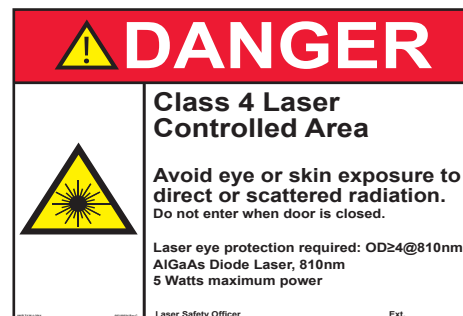
Figure 42 - Danger - Laser signage
