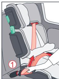
Pass the lap section of the adult belt through the red lap belt guides on each side of the hifold ②.
