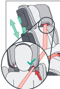
8. Pass the diagonal belt across the child's body and allow the diagonal belt to pass over the outside of the base side panel belt guide ①.
