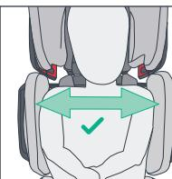
4. Adjust the width of the Headrest Sides so they are close to child's head. See instructions in "Preparing for Use" section.
