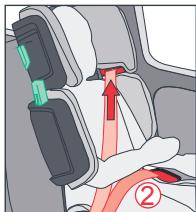
9. Check that vehicle lap belt is supported on pelvis such that the belt is low on hips and contacting thighs and that there is no slack or twists in the seat belt.
