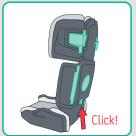
On the backrest side panel the seat back fold locking button should project above the top of the side panel and be locked.
