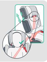
Check that vehicle lap belt is supported on pelvis such that the belt is low on hips and contacting thighs and that there is no slack or twists in the seat belt.
