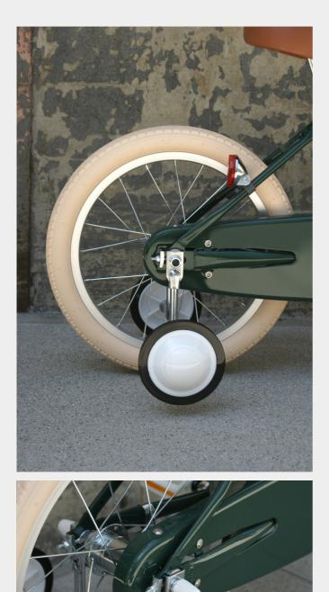
With a 15mm wrench, remove the pre-installed axle bolts and washers before installing the arm and stabilizer onto the bicycle. Axle bolts may be very tightly secured on the frame. This is normal, keep trying!
