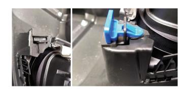
**Step 2:** To assemble the Quattro, attach the bracket using the supplied carriage bolt, washer and tighten the bolt until it's snug but not fully tight. The kit includes two thicknesses of sticky back EPDM, which is intended to be placed onto the brackets' tabs labeled 1 & 2. For the Tundra, cut the **THICK** EPDM into  $\frac{1}{2}$ " x  $\frac{1}{2}$ " squares and place it onto the tabs' backside.
