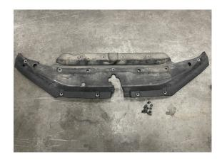
After removing the factory fog light, take note of the two slots on the inner side. These will be used when installing the Quattro. Some models come with a protective shroud protecting the backside of the fog light. You can remove the covering by releasing the two pressure tabs on each side, followed by pressing downward on the top to release the top hook.
