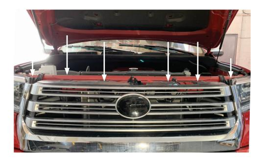
**Step 2:** If equipped with the front parking sensor, unplug the harness located beneath the panel on top of the grille.
