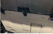
**Step 5:** With the fascia removed, locate the six 14mm frame bolts, three on each side. These bolts will be removed and reinstalled after the light bar bracket.
