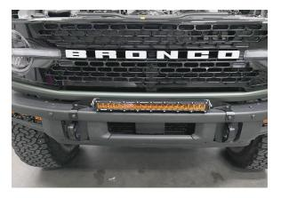
**Step 2:** Route the wiring harness. With the light bar installed, route the end of the harness with the plug down behind the driver side headlight and the over to the light bar harness. Be careful to avoid any hot, sharp, or moving objects.
