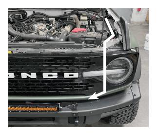
Continue routing the wiring harness toward the fire wall zip tying the harness along the way. The Upfitter auxiliary wires are bundled up on the harness that runs along the firewall.
