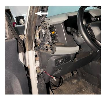
Next, pull the seal that runs up the A- pillar, remove the trim covering the roof latch, and remove the trim panel that covers the air bag. Taking off the driver side roof might be necessary to get the latch cover off, due to the stiffness of the clips. The air bag trim panels are held in by five 8mm bolts that will need to be removed. Once all of the panels are removed, route the wire up the A-pillar, keeping the wire behind the air bag.
