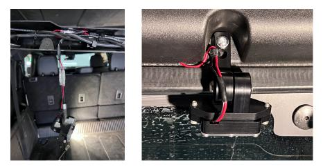
**Step 5:** Connecting the power. To supply constant power to the lights the on and off switch will need to be cut off. Cut the switch as indicated in the diagram and connect the 2 red wires together using the barrel connector.
