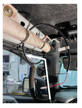
With the wires run, connect the one of the "Y Splitters" to the "84 Inch Extension" followed by the dome light and one of the "42 Inch Extensions." Route the "42 Inch Extension" toward the rear keeping the wire behind the air bag. Connect the rear interior light using another "Y Splitter" followed by an "84 Inch Extension" and route the wire down the B pillar and back towards the rear cargo area.
