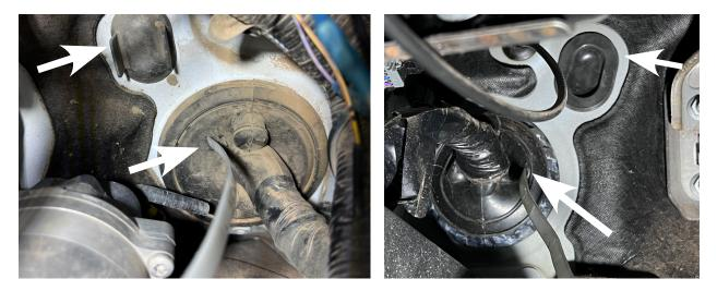
**Step 3:** With the wires ran through the firewall, the next step is to route them to the back of the vehicle. The door seal panel and dash handle will need to removed.
