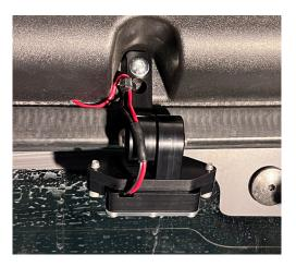
**Step 5:** Connecting the power. To supply constant power to the lights the on and off switch will need to be cut off. Cut the switch as indicated in the diagram and connect the 2 red wires together using the barrel connector.
