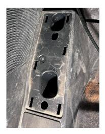
Remove the rear bottom door seal panel by pulling upward towards the roof and route the wire as indicated in the image. The b-pillar panel does not need to be removed, the wire can be "tucked" underneath.
