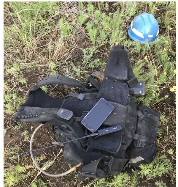
Figure 1— goTenna Pro and phone running ATAK
