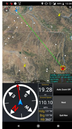
Figure 6—Navigating to an initial attack fire (note pushpins for WildCAD incidents and white dots for lightning strikes)
