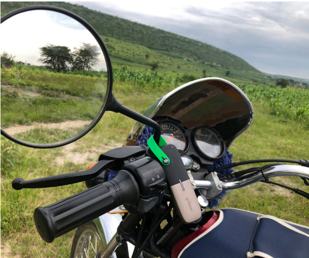
Rafael Muvunga attaches the goTenna Mesh to his motorcycle to enable off grid communication with his colleague
