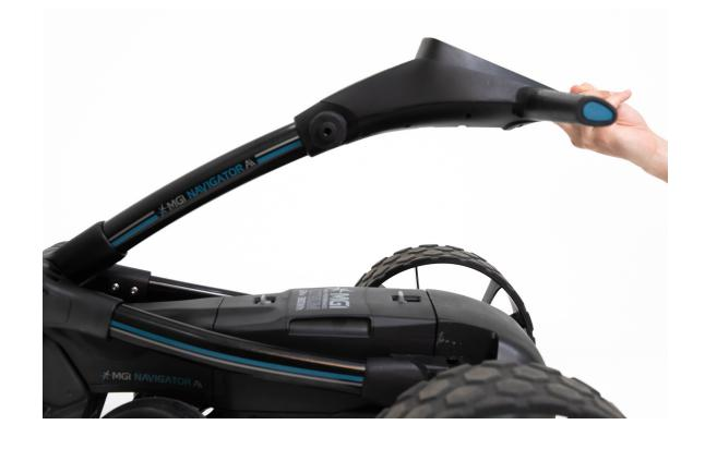
STEP 3: Lower handlebar until touching chassis.
