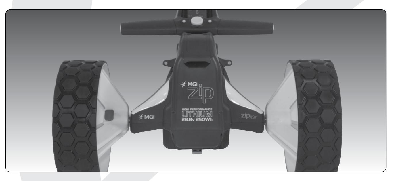
On the wheel, press the grey release button on the wheel hub. Place the wheel onto the axle. You will notice you need to match up the inner female groove on the axle and the male of the wheel. When placed in position simply release the button. You will notice you hear a "click" when the wheel is properly secured. To check that the wheel is properly in position pull
