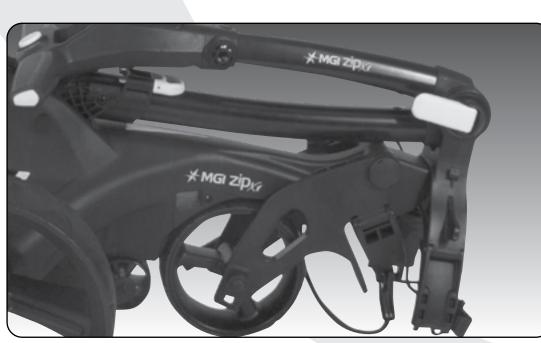
**Step 5:** Push the toggle down on the top bag support and then move the Top Bag Support down so that it locks over the front wheel assembly.
