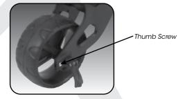
Roll the left or right hand side silver thumb screw UP to straighten the Zip X4 more to the LEFT.
