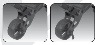
**Step 2:** There are two silver thumb screws located on either side of the front wheel. Adjusting these screws will help straighten the alignment by correcting the Zip X4 to track more to the left or the right.
