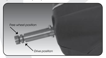
i. Drive position - Lock the wheel onto the groove closest to the battery base. To do this, press the grey release button on the wheel hub, push the wheel on to the axle as far as possible. To test for drive position try rolling the wheel backwards. If you feel resistance then the wheel is now in drive position and ready to use. Repeat for both wheels.
