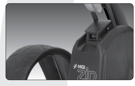
**Step 1:** Disconnect the battery by lifting the battery handle. It can be left on or removed from the Zip Navigator AT.
