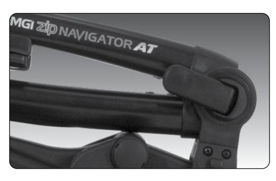
**Step 6:** Close the fold lever to lock the handle into place.
