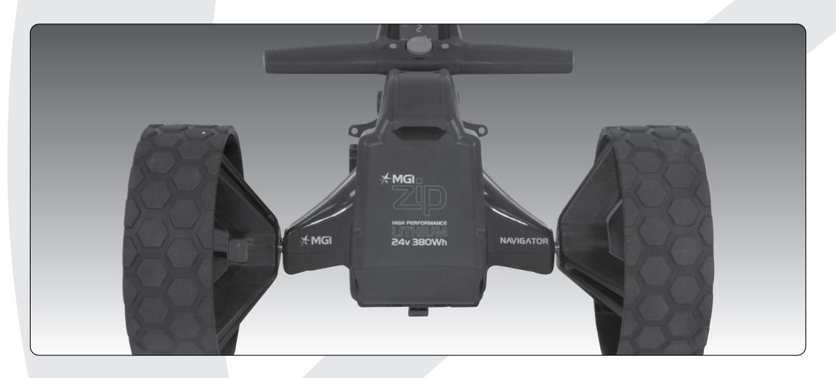
Press the grey release button on the wheel hub. Place the wheel onto the axle. You will need to match up the inner female groove on the axle and the male of the wheel. When placed in position simply release the button. You hear a "click" when the wheel is properly secured. To check that the wheel is properly in position pull on the wheel. If it is properly in position it will not slide off. Repeat for the other wheel.
