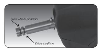
i. Drive position - Lock the wheel onto the groove closest to the battery base. To do this, press the grey release button on the wheel hub, push the wheel on to the axle as far as possible. To test for drive position try rolling the wheel backwards. If you feel resistance then the wheel is now in drive position and ready to use. Repeat for both wheels.
