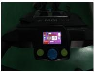
3. Turn the speed button clockwise, the counter on the Navigator Quad ITB PCB display will increase from R 01 to R 50 as below left two pictures. Turn the speed button anti clockwise, the display will reduce from R 50 to 00 and then increase from L 01 to L50 as the right picture. R50 means to adjust the buggy to turn right for 50 units. R09 means to adjust the buggy to turn left for 50 units. L05 means to adjust the buggy to turn left for 5 units and so on.
