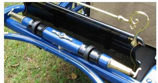
Brass wear plate mounted on top of the singletree to support the bolt.
