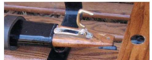
Trace holder incorrectly left up.
