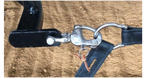
This metal singletree requires snap shackles and ring end traces.
