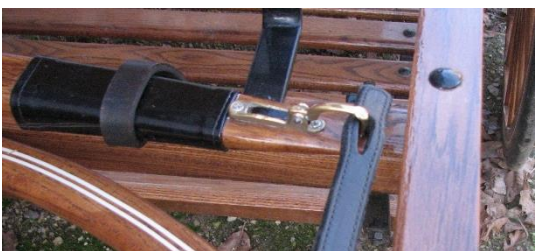
Trace attached incorrectly. The hardware WILL break if the trace is attached this way.
