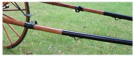
If your shafts are metal, it becomes a little more complicated. The footman loops are generally welded on metal shafts. Depending on the composition of the metal, footman loops may be screwed on the shafts, but otherwise you will have to find a good welder to attach new loops.
