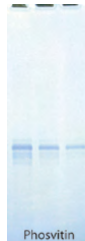
Figure 25: Various concentrations of phosphoprotein were loaded onto the FOCUS™ PhosphoRich™ columns and were washed extensively. The protein was rapidly eluted and the eluted proteins were resolved by SDS-PAGE. The phosvitin was visualized with the Reversible Zinc Stain™.
