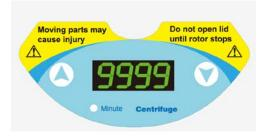
Use the up and down arrows to adjust the timer setting. The timer range is 1 second to 9999min.
