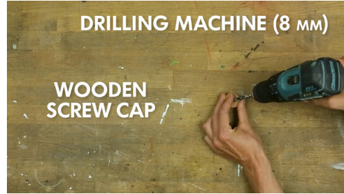
10. Drill a hole into the wooden screw cap.
