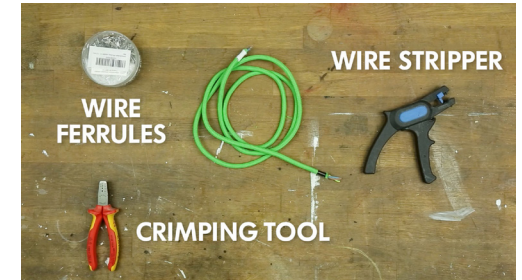
4. Afterwards you need the crimping tool, the wire stripper and wire ferrules.
