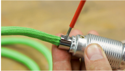
9. Screw the E14 socket in tight.
