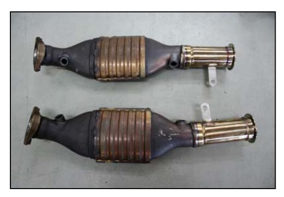
Completed STUBBIES to the BMW factory catalysts ready to be installed for street use
