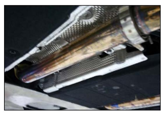
FRONT section of the Active Autowerke X-PIPE installed for race prep
