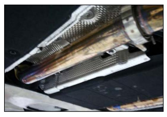
Remove the front pipes of the X-PIPE and install the cut off factory catalyst.
