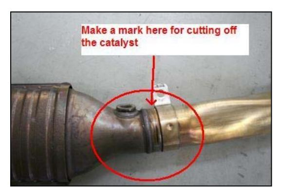
On the LEFT catalyst, there is a weld mark made by the factory. Approximately 10mm after the weld, there is a depression. Using a felt tip marker, make a mark all-around as a guide mark.
