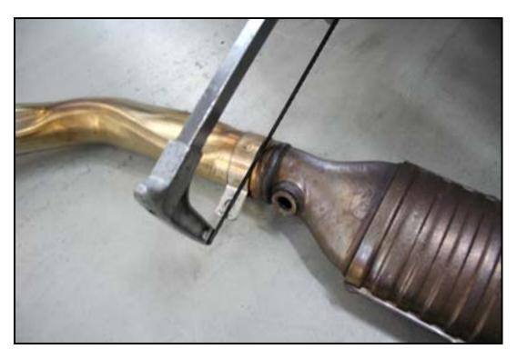
Using a hack-saw, cut off the LEFT catalyst
