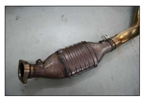
Picture of the LEFT side catalyst and the mark to be made for cutting off the catalyst
