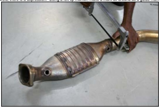
Using a hack-saw, cut off the RIGHT catalyst
