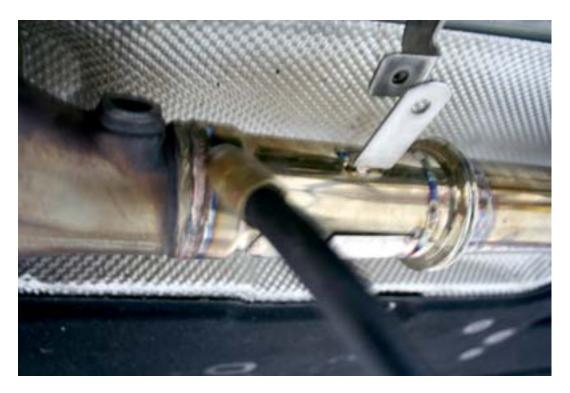
Position the STUBBIE between the factory catalyst and the Active X-PIPE and secure with the V-BAND clamp and other mounting hardware. The Stubbies have a sleeve making the pipes slide on for a partial fit.
