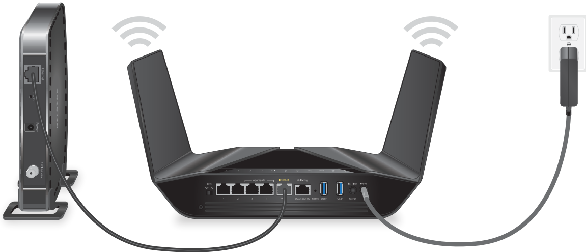
Figure 6. Cable your router
