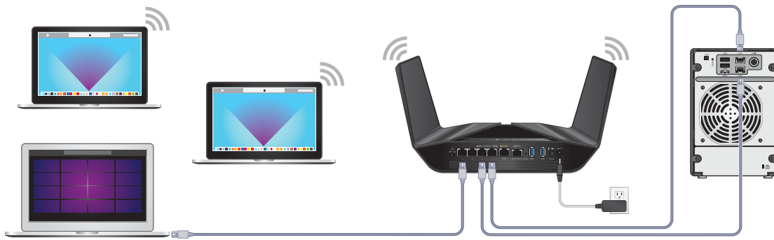
Figure 7. Ethernet port aggregation to a LAN device
