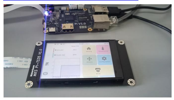
Web page control: When MKS PI is connected to a router, the corresponding IP can be displayed on the screen (if there is no router, you can query the corresponding IP in the router). Then you can enter the corresponding IP in the browser on the PC on the same router network to enter the FLUIDD control interface to control
