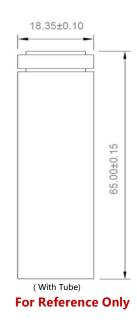
(1) CC-CV, 1.25A to 4.2V, 100mA cut-off at 25°C; CC, 0.5A to 2.5V cut-off at 25°C.
