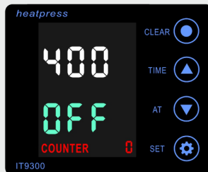
Heat press enters into power off mode if machine is kept quietly for set time and without any operation
