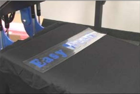
**6** Now position the EasyWeed application on the garment. If your heat press has a built in timer, set it for 10-15 seconds. Place the Teflon sheet over the graphic, then close the heat press. After 10-15 seconds, open the press.
