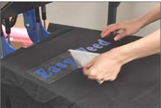
**7** You do NOT have to allow the garment to cool to room temperature before removing the release liner. This is a hot peel product. Slowly peel the release liner away from the shirt. The garment film should remain on the fabric resulting in an image with a soft feel.
