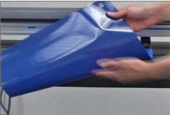
**1** When using Siser EasyWeed, you will notice that the release liner is completely clear. When you cut, load the glossy side downwards into your cutter, allowing the opaque side to be facing upwards.
