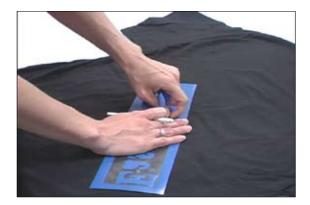
Your plotter will cut a mirror image of the original design into the garment film. When the cut-job is complete, advance the material forward and remove from the cutter using the Xacto, Olfa, or other utility or hobby knife. Using your preferred weeding tool, weed the excess material from the release liner. You will find that it is indeed very easy to weed.
