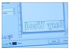
2 After designing your graphic, click the send to plotter button. Verify proper film sizing, then click your "reverse image", "mirror" or "flip" icon. This will reverse the image on your screen and allow for image reversal when cutting. For this tutorial, we are using Vinyl Express LXi. The reverse icon in Vinyl Express LXi is an F, for "flip".
