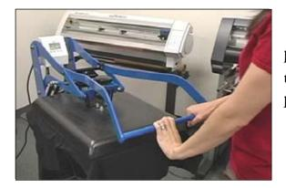
5 You must preheat the garment before applying the Easy-Weed. Adjust the heat setting to 302° F. If your heat press has a built in timer, set it for 4 seconds. Place the garment on the heat press. Close the heat press. After 4 seconds, open the press.
