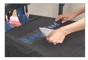
You do NOT have to allow the garment to cool to room temperature before removing the release liner. This is a hot peel product. Slowly peel the release liner away from the shirt. The garment film should remain on the fabric resulting in an image with a soft feel.
