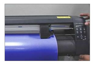
3 Next load media into the cutter. Make sure to load the media with the glossy side facing down and the opaque side facing up. After loading the film and setting the proper cutting conditions on your plotter, perform a test cut to make sure you have proper blade depth and a weedable graphic. For cutting SISER EasyWeed, we suggest a standard 45° blade at about 70 grams of force. After you have performed a satisfactory test cut, send the job from your sign making software.
