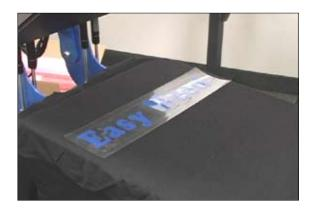
6 Now position the EasyWeed application on the garment. 6 If your heat press has a built in timer, set it for 10-15 seconds. Place the Teflon sheet over the graphic, then close the heat press. After 10-15 seconds, open the press.
