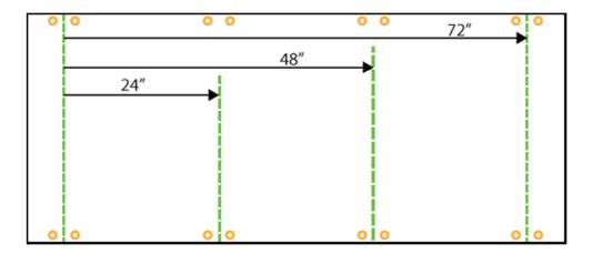
Media should always be cut halfway between the two closely spaced grommets.
