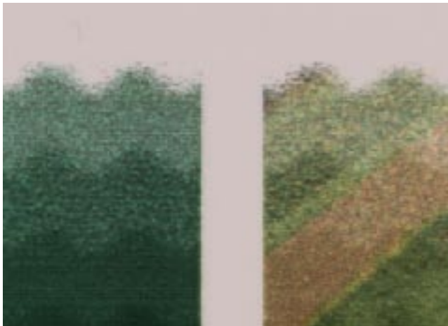
In the FLAAR+BGSU lab, using the QEA instrument, and 80-megapixel scan from the Cruse, you can see the weaving pattern at the left, and the other pattern at the right. One pattern is for “pictures” (the waves); the other pattern is for large areas of dark colors (“signs”). Please understand, this is a cross-section of a deliberately unfinished weave, to reveal the pattern before it is finished. The purpose is to show that there are two forms of the pattern.
