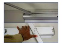
**Step 2:** Remove the pin in the right side of the case and pull the carrier sheet upward to expose the instructions and strip of adhesive tape. Reinsert the pin to lock the sheet in this position.
