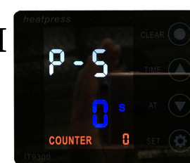
P-5: Pre-alarm setting
