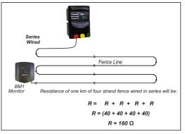
Series wiring results in one long wire, thereby increasing the resistance of the fence. This circuit is generally used for security fencing. Short out any wire and the monitor will trigger an alarm.
