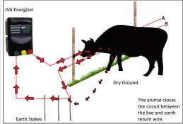
Dry ground is a poor conductor of electricity. In this circuit one adds an earth return wire (B) to the fence. The animal now closes the circuit between the live wire (A) and earth return wire (B) and so one does not rely on the poorly conductive, dry ground to close the circuit.
