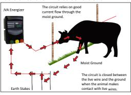
Moist ground is a good conductor of electricity, so in this circuit the electricity will flow from the Energizer, along the wire, through the animal closing the circuit, back through the ground to earth electrodes and on up into the energizer, thereby completing the circuit and delivering the shock.
