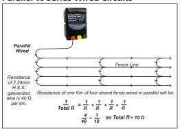
Parallel wiring reduces the resistance of the fence line, thereby enabling it to deliver a more powerful shock but it is less sensitive to shorting. This makes it more suitable for livestock control but less suitable for security fences.
