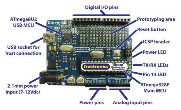
The Freetronics Eleven is a microcontroller board which is 100% compatible with the popular Arduino Uno reference design, while incorporating several updates and improvements.
