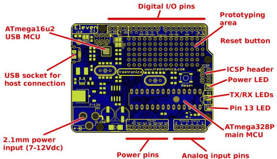
All I/O pins and power rails are brought out to convenient headers, allowing you to either connect individual pins to a breadboard using standard jumper wires or to plug in "shield" daughter-boards for versatile expansion. General-purpose prototyping shields are also available which provide extensive space for you to create your own add-on circuits.
