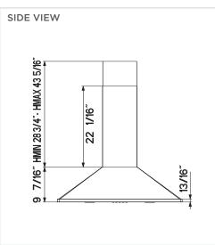
Ducted/Ductless with DUCTCLPL Top 6" Round
