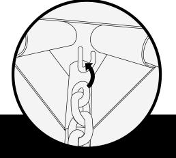
Attach the chain to the hook under the cap to set cauldron at desired height.
