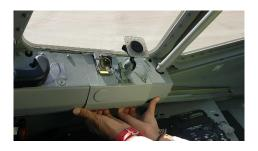
While pulling the edge, gently lift the device upwards.
