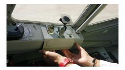
Continue lifting the device upwards with both ends, while maintaining clearance from the clip.
