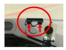
Lift the forward chart spring clip up. Slide the device out from underneath the raised chart spring clip. Lower the clip once the device is clear.
