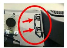
Raise the outboard chart spring clip. Rotate the device so the outboard edge of the device is flush against the raised clip housing. Lower the clip to capture the 2 vertical tabs on the outboard edge of the device.
