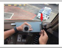
With your other hand, lift the lower edge of the device to remove it from the chart table.
