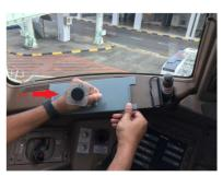
While pushing the device forward, raise the chart spring clip.
