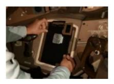
Slide device off the Lunchbox door, lower the chart spring clip (if installed) and close the door.
