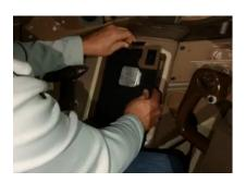
Lower the chart spring clip (if installed) so it rests on top of the device.
