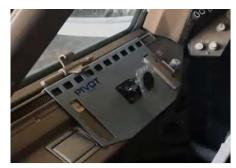
With one hand, raise the chart spring clip. Using your other hand, slide the device aft to remove the chart spring clip from the slot in the device.
