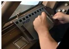
With the other hand, lift up on the device to separate it from the gap in the window shade channel.
