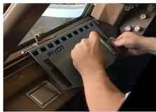
Release chart spring clip. Press down on the top edge of the device to secure it in position. Raise the window shade to ensure there is no interference with its operation.
