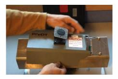
Keep lowering until the bottom of the inboard edge of the device snaps into place in the gap between the window shroud and the sidewall.
