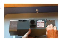
Pull inward on the tab in the center of the device to clear the bottom of the window shroud.
