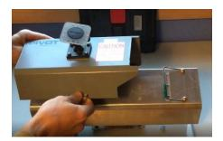
Lower the device onto the window shroud and rotate it slightly forward toward the chart spring clip.
