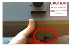
Lift upward until the device pops off the window shroud.
