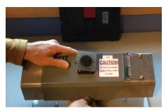
Lift the chart spring clip and push the unit forward until the raised tab on the device is captured by the chart spring clip.
