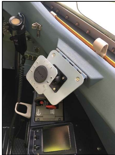
Figure 1 PM-ATR-X Installed on First Officer's Side
