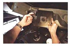
With the device fully forward, release the chart spring clip as shown.
