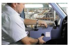
Slide the device under the raised chart spring clip and place the top edge of the device over the window shroud
