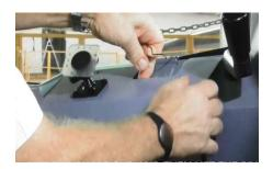
Once it is separated from the window shroud, lift the edge away from the window shade slot.
