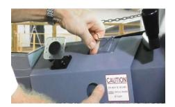
Using your other hand, lift the forward portion of the device to lift the top edge away from the window shroud.
