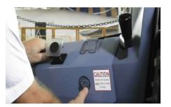
Press down and clip the lower edge of the device onto the window shroud until the unit snaps into place.
