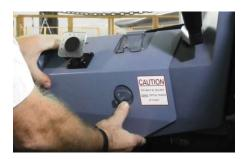
Adjust tension on mounting plate to the appropriate level.
